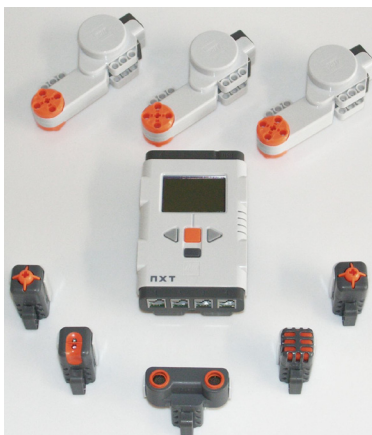
Fig. 1. LEGO Mindstorms NXT hardware of the standard education kit: Five sensors (light, sound, ultrasonic, and two touch sensors), three servo motors, and the programmable NXT intelligent brick.
